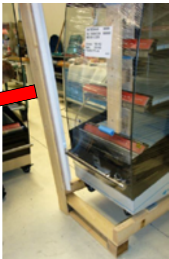
Remove vertical beams and protection on front side
