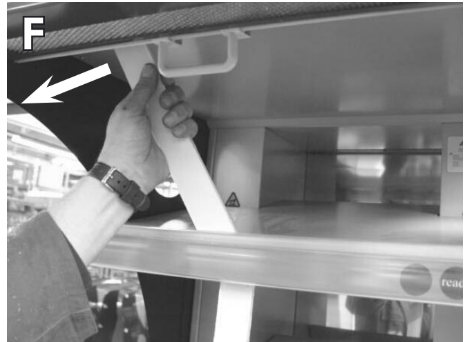
Remove top transport safety beam
