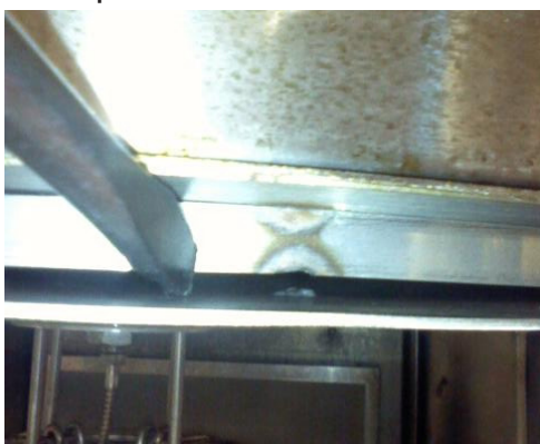
Example of broken weld
