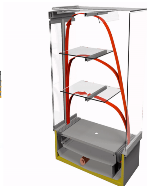
Hot air flow Full Serve
