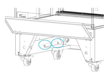
Place bracket into mounting position and fasten with 4 mounting bolts.
