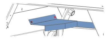
Place bracket into mounting position as seen on drawing
