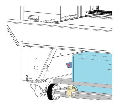
After mounting, the waste water trolley can be placed in position.
